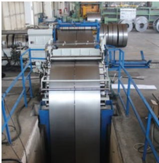
SHEET METAL SLICING LINE
